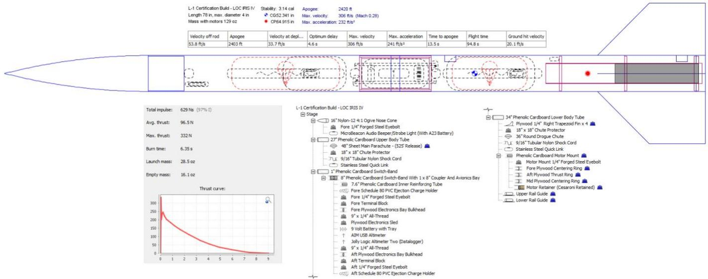
Dimensions and Design of Removable-Cap Nylon-12 3D Printed Nose Cone for LOC IRIS IV L-1 Build:
