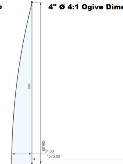
**Proposed Nose Cone for L1 Certification Build (IRIS.) 4" Ø by 20" Length Cap-To-Tip Nose Cone with Perfect 4:1 Ogive Printed Using Nylon-12 Polymer ((C12H23NO)n.)**
