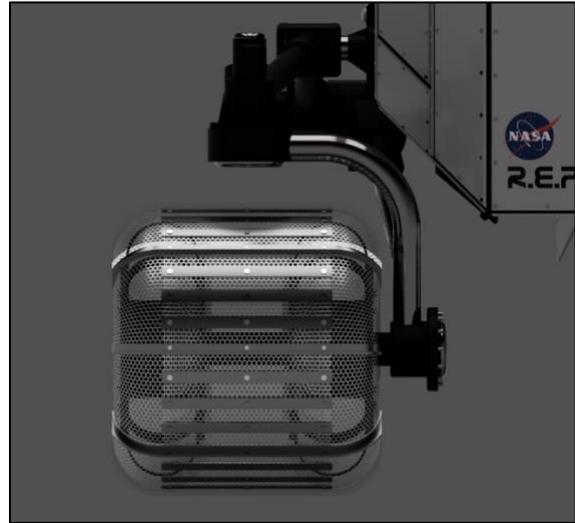
*Figure 1- Oblique view of the double torus design wheel assembly. (Note the negative deflection bars mounted internally.)*
