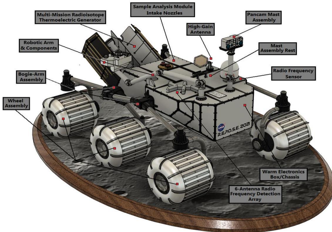
Figure 3 - Oblique model of REPOSE Lunar Rover with external labels.
