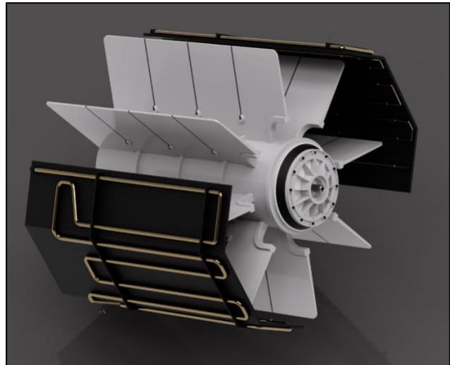
*Figure 4 – B-Field Magnetic Spectrometer with aluminum mounting bracket.*
