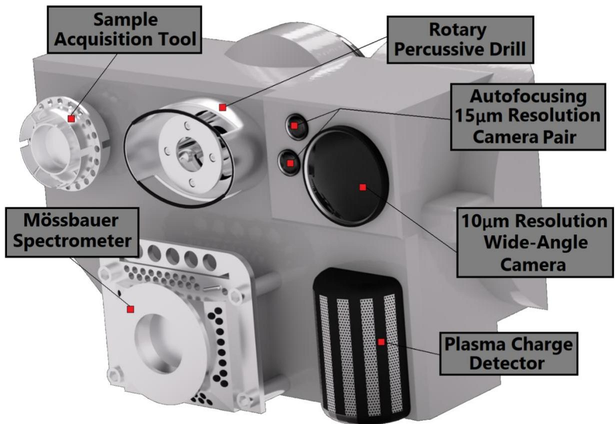
Figure 6 – Robotic Tool/Turret/Hand with multiple tool labels.
